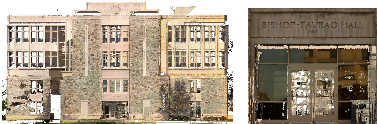
Fig. 16. Details of the terrestrial laser scanner-based Point cloud (Left: south façade; Right: main entrance door).
